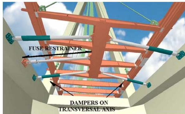
Fig. 8 Dissipation system between deck and piers
